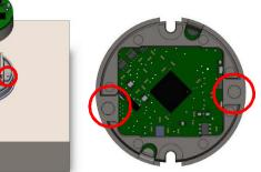
Insert two M2 screws with washers and lock washers and tighten using a Torx T6 key with a torque of 35.4 oz-in.
