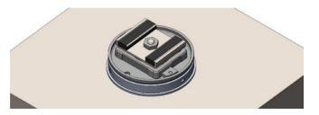
Align PCB with carrier to frame (two different keys) and push down until it locks into place.
