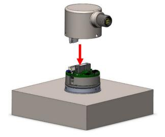
Slide housing over adapter plate. Be careful to not pinch cable. Secure housing by tightening the three M2.5 screws using a Philips screw driver with a torque of 56.6 oz-in.
